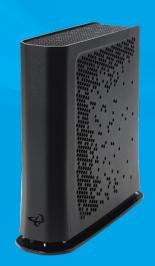
The ARIA3411 is packed with features that make it the ultimate home networking solution. With its multi-gigabit wired backhaul, you can enjoy maximum speeds and a rock-solid connection for all your connected devices. The Extender/Router boasts three Ethernet ports - two 1-Gigabit WAN LAN ports and one 2.5 Gigabit WAN port - providing Gigabit speeds to all your devices.
