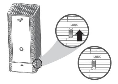
Install the battery by opening up the door under the module, aligning it in the proper direction and then closing the door once more.
